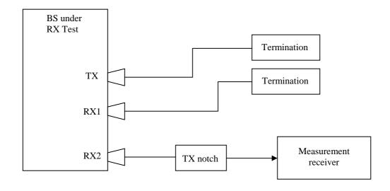
Figure I.2-6: Measuring system Set-up for Receiver spurious emission
