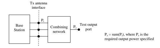
Figure 4.5.7.2-1: Transmitter test set-up
