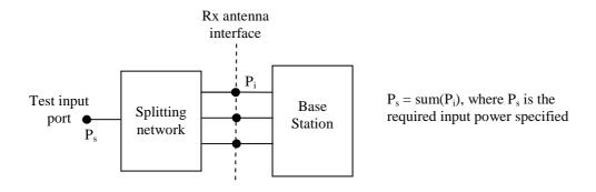
Figure 4.5.7.1-1: Receiver test set-up
