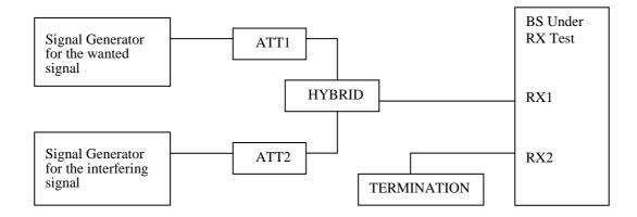
Figure I.2-4: Measuring system Set-up for Adjacent channel selectivity and narrowband blocking
