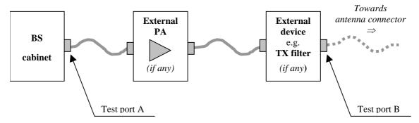
Figure 4.5-1: Transmitter test ports
