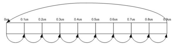
Figure 8.4.1.4.2-2 Timing offset scheme
