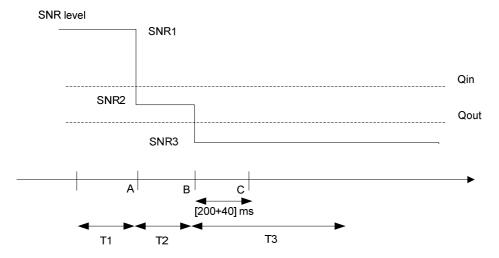
Figure A.7.3.9.1-1 SNR variation for out-of-sync testing
