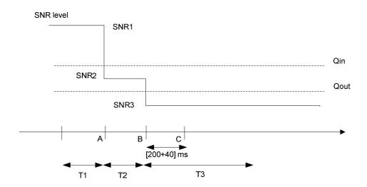
Figure A.7.3.1.1-1 SNR variation for out-of-sync testing
