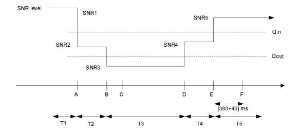
Figure A.7.3.4.1-1. SNR variation for in-sync testing
