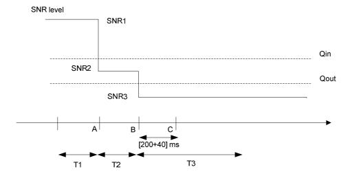
Figure A.7.3.3.1-1. SNR variation for out-of-sync testing
