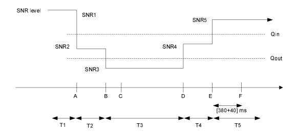
Figure A.7.3.2.1-1 SNR variation for in-sync testing
