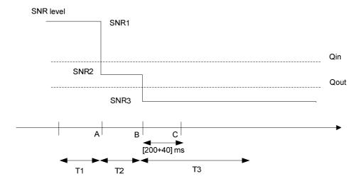
Figure A.7.3.14.1-1 SNR variation for out-of-sync testing
