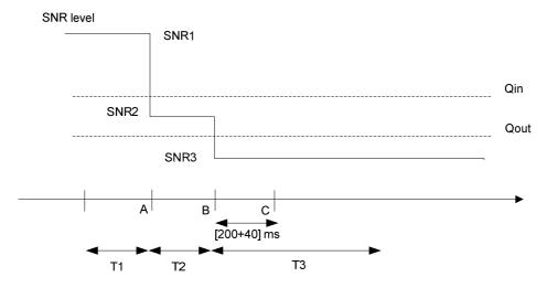
Figure A.7.3.13.1-1 SNR variation for out-of-sync testing
