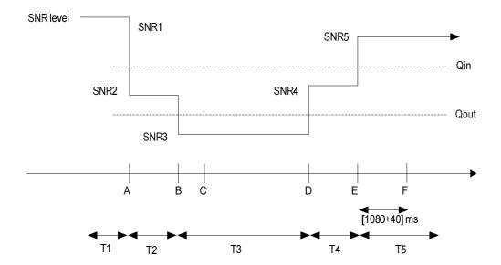
Figure A.7.3.8.1-1 SNR variation for in-sync testing in DRX
