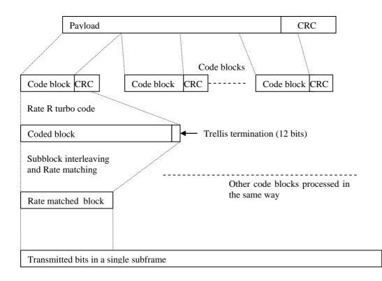
Figure A-1. Schematic overview of the encoding process
