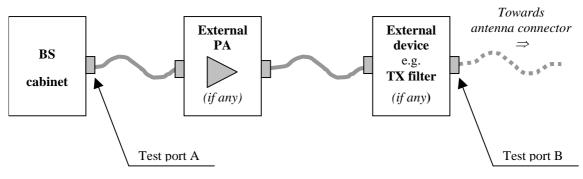
Figure 6.1-1: Transmitter test ports
