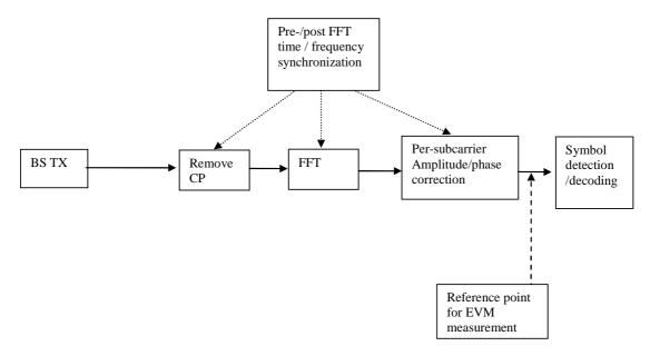
Figure E.1-1: Reference point for EVM measurement
