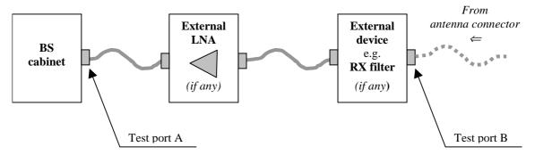
Figure 7.1: Receiver test ports
