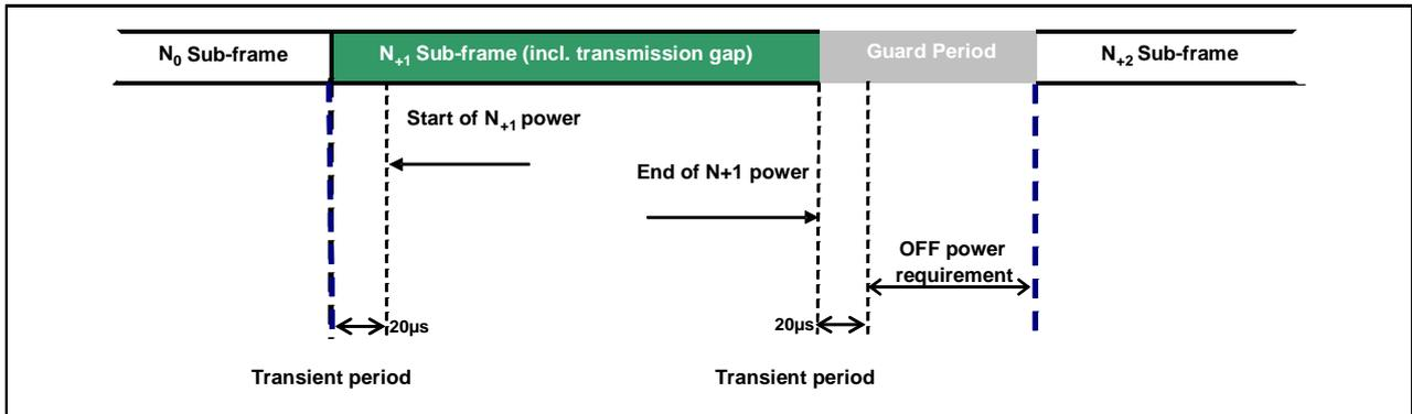
Figure 6.3.4D.1-1: PSDCH/PSCCH/PSSCH time mask
