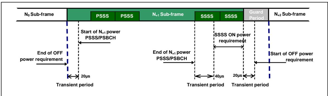
Figure 6.3.4D.3-1: PSSS/SSSS/PSBCH time mask for normal CP transmission
