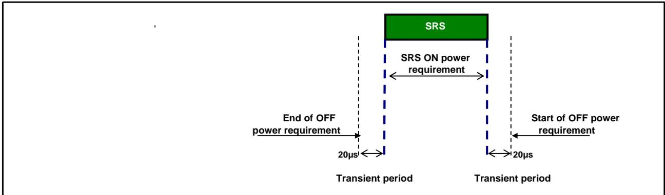
Figure 6.3.4.2.2-1: Single SRS time mask
