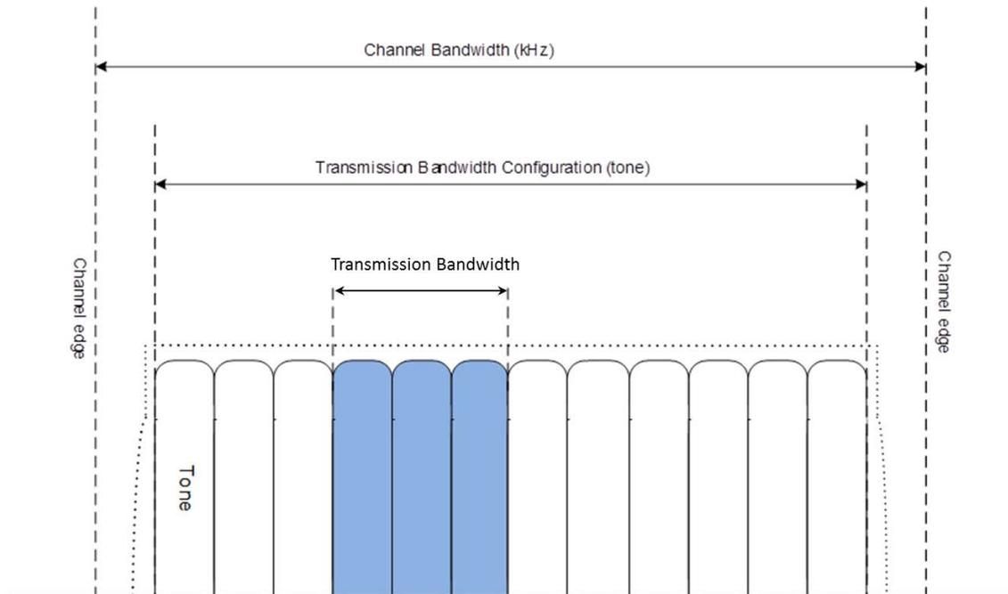
Figure 5.6F-1 Definition of Channel Bandwidth and Transmission Bandwidth configuration
