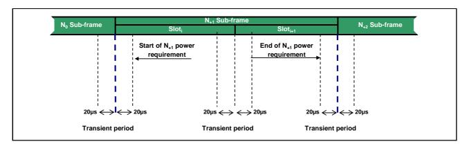
Figure 6.3.4.3-1: Transmission power template
