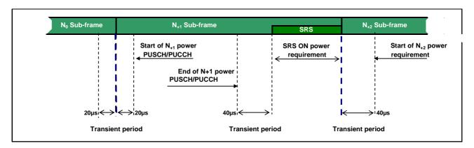
Figure 6.3.4.4-2: PUCCH/PUSCH/SRS time mask when there is transmission before and after SRS
