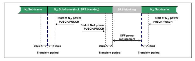
Figure 6.3.4.4-4: SRS time mask when there is FDD SRS blanking
