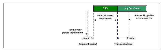
Figure 6.3.4.4-3: PUCCH/PUSCH/SRS time mask when there is a transmission after SRS but not before
