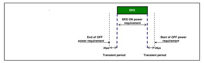
Figure 6.3.4.2.2-1: Single SRS time mask
