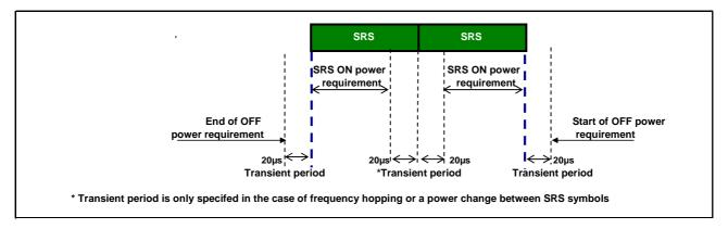
Figure 6.3.4.2.2-2: Dual SRS time mask for the case of UpPTS transmissions
