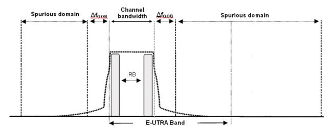
Figure 6.6-1: Transmitter RF spectrum
