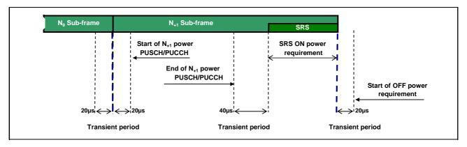
Figure 6.3.4.4-1: PUCCH/PUSCH/SRS time mask when there is a transmission before SRS but not after
