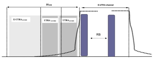
Figure 6.6.2.3-1: Adjacent Channel Leakage requirements for one E-UTRA carrier
