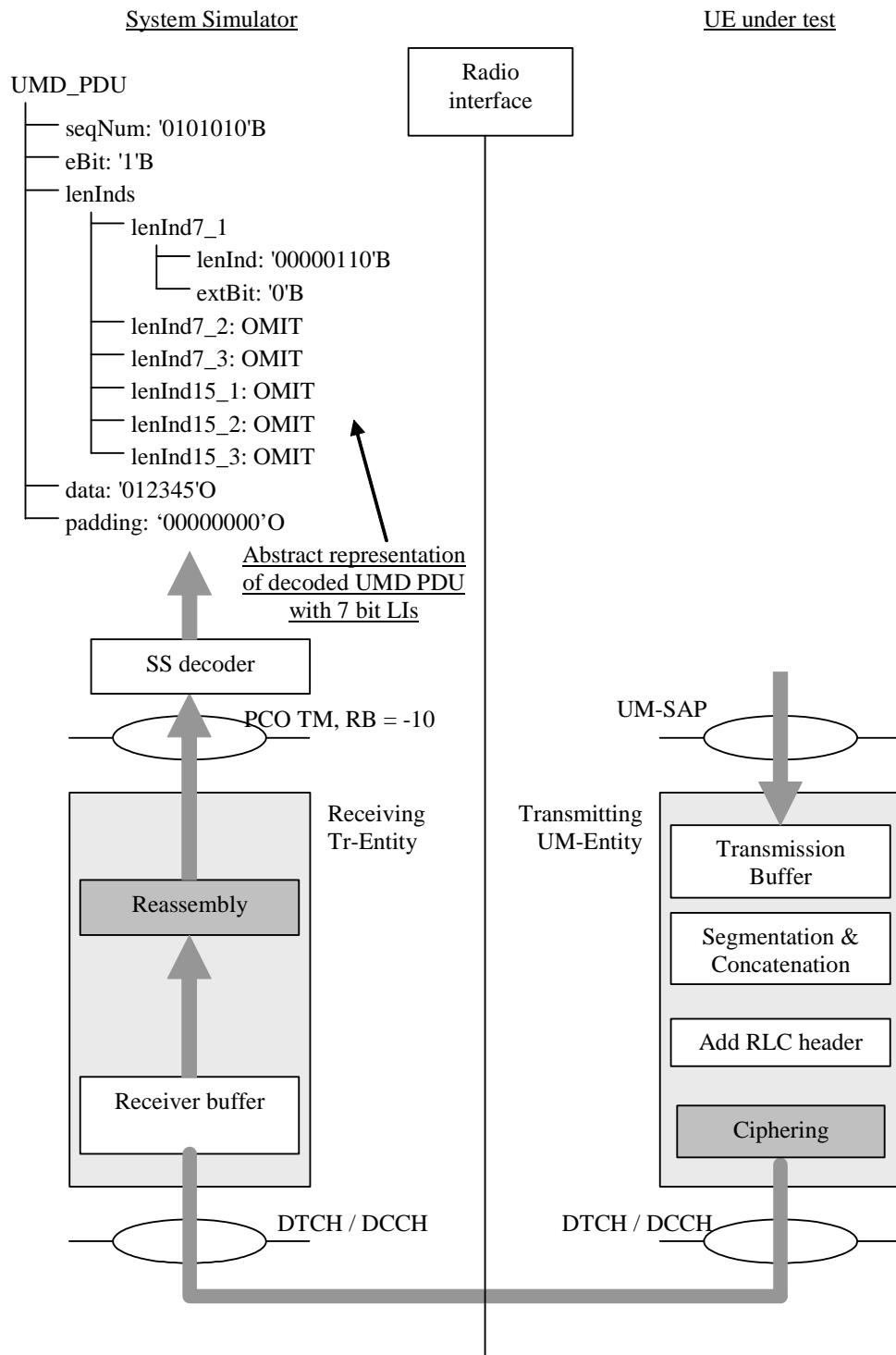
**Figure 6.5.2.2: Example configuration for uplink RLC UM testing**
