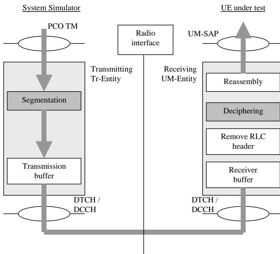
**Figure 6.5.2.1: Example configuration for downlink RLC UM testing**
