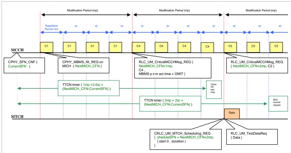
**Figure 8.14.2.1: Synchronized MTCH data sending, no MSCH configured**
