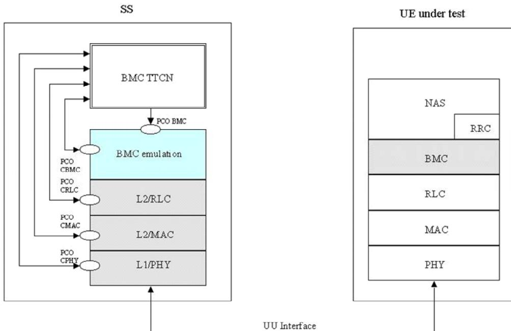
**Figure 6.8: BMC testing architecture single party method**
