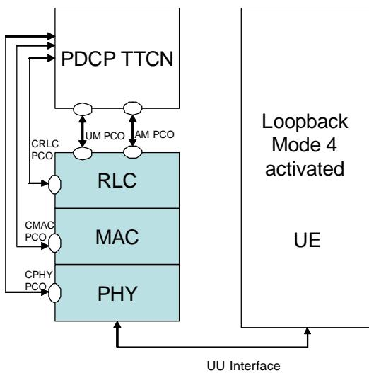
**Figure 6.9.2.2: Network initiated secondary PDP testing architecture**
