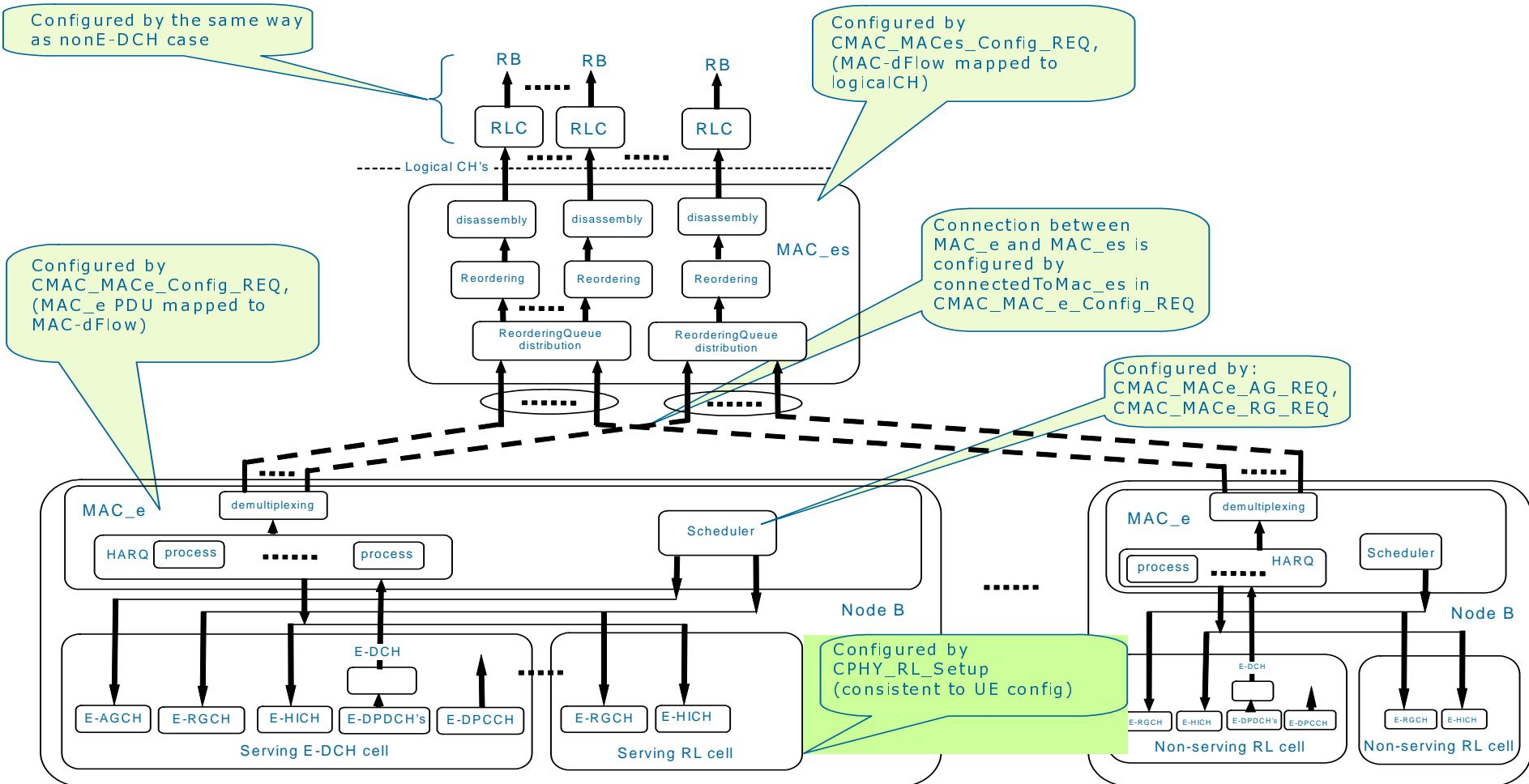
Figure 6.13.1: The model of E-DCH testing with MAC-e/MAC-es
