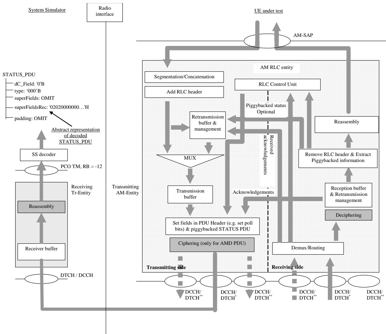
**Figure 6.5.2.3: Example configuration for uplink RLC AM testing**
