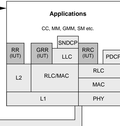
Figure 6.10.2.9.6: The model of multi-RAT handover testing
