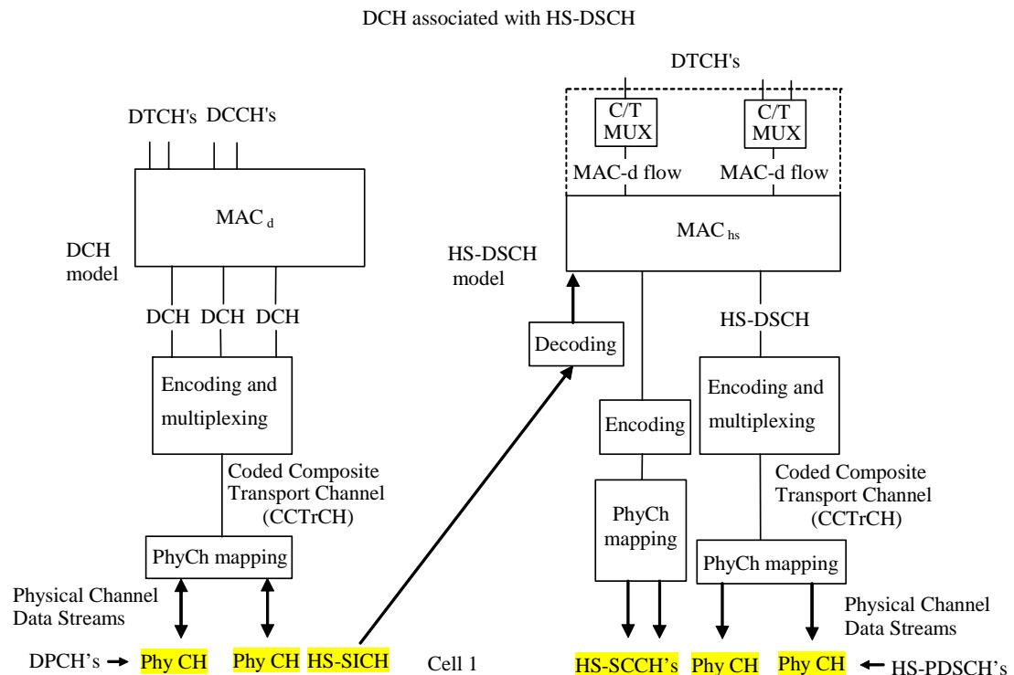
**Figure 6.12a: Associated DCH with HS-DSCH model for 1.28 Mcps TDD**
