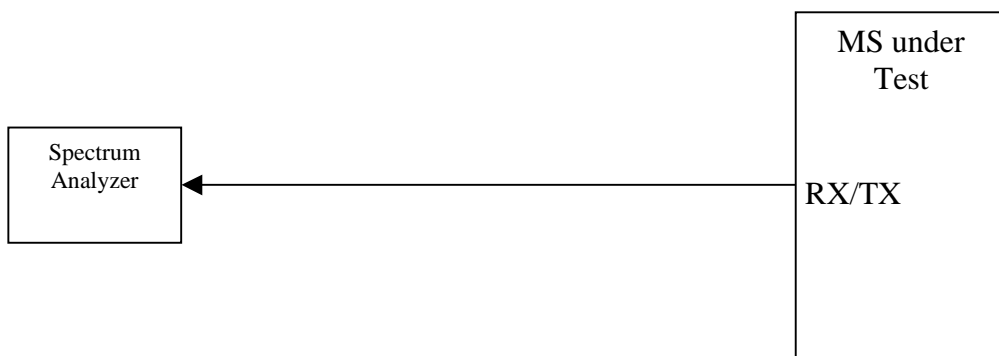
Figure A.8: Connection for Spurious Emission Test
