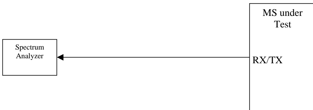
Figure A.8: Connection for Spurious Emission Test
