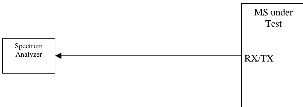
Figure A.8: Connection for Spurious Emission Test
