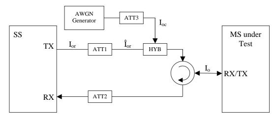
Figure A.9: Connection for Static Channel Test
