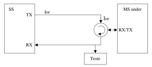
Figure A.1: Connection for Basic TX Test
