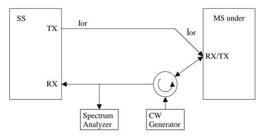
Figure A.2: Connection for TX Intermodulation Test
