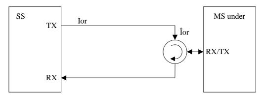
Figure A.3: Connection for Basic RX Test
