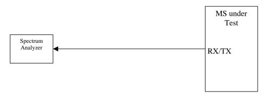
**Figure A.8: Connection for Spurious Emission Test**
