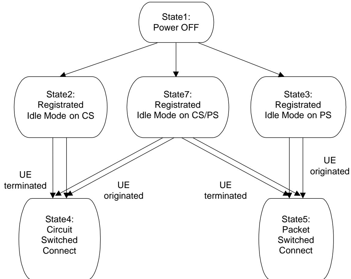
Figure 7.2.1.1: UE Test States for Generic setup procedures
