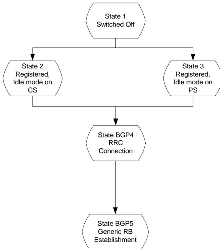
**Figure 7.1.1: UE Test States for Basic Generic Procedures**
