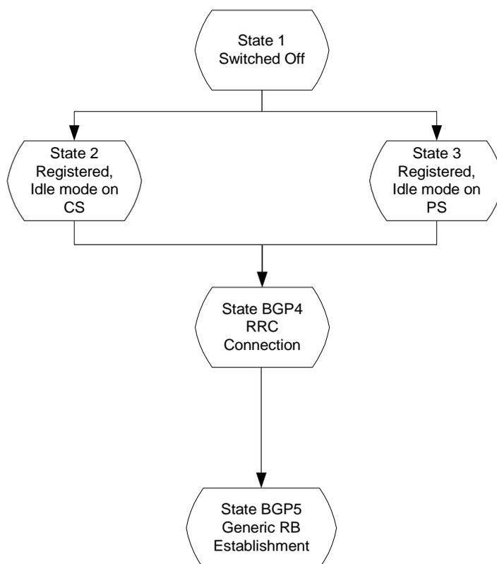
**Figure 7.1.1: UE Test States for Basic Generic Procedures**
