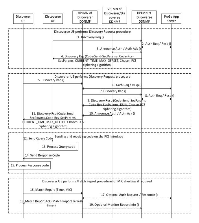
Figure 6.1.3.2.2.2-1: Security procedure for restricted 5G ProSe Direct Discovery Model B
