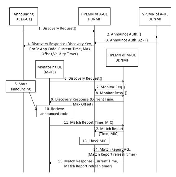
Figure 6.1.3.1-1: Open 5G ProSe Direct Discovery security procedure
