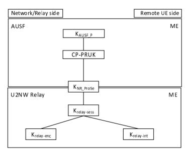
Figure 6.3.3.3.1: PC5 Key Hierarchy for 5G ProSe UE-to-Network Relay security over Control Plane
