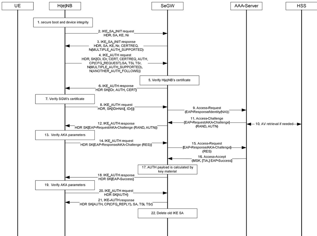
**Figure A.2: Combined certificate and EAP-AKA-based authentication**
