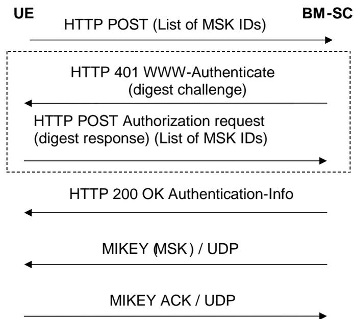
**Figure 6.1: Basic MSK retrieval procedure**
