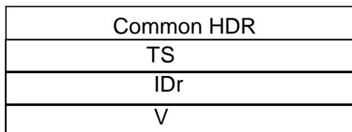
**Figure 6.6: The logical structure of the MIKEY Verification message**
