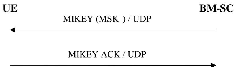
**Figure 6.3: Pushing the MSKs to the UE**
