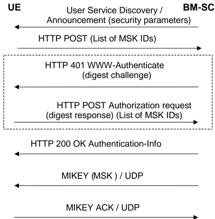
**Figure 6.2a: MSK retrieval procedure**
