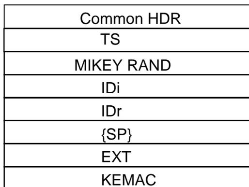
**Figure 6.5: The logical structure of the MIKEY message used to deliver MSK.
