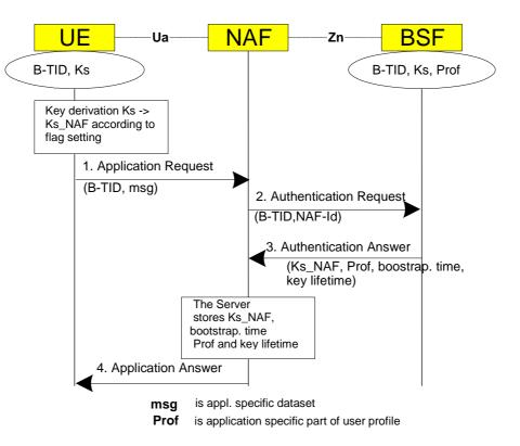
Figure M.3: The bootstrapping usage procedure
