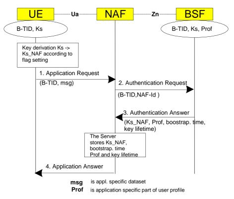
Figure 4.4: The bootstrapping usage procedure
