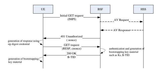
Figure M.2 GBA\_Digest bootstrapping procedure
