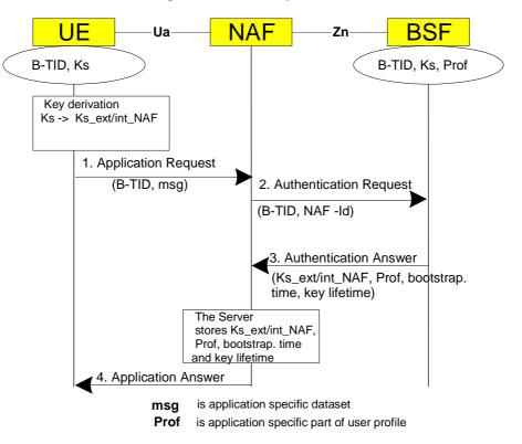
Figure 5.3: The bootstrapping usage procedure with UICC-based enhancements
