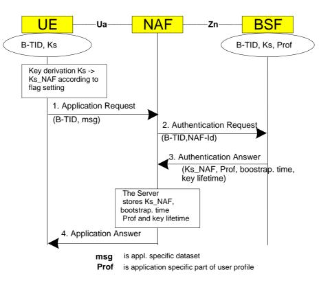
Figure I.4: The bootstrapping usage procedure
