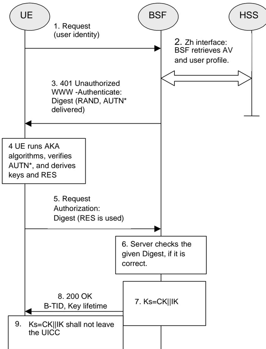
**Figure 5.1: The bootstrapping procedure with UICC-based enhancements**
