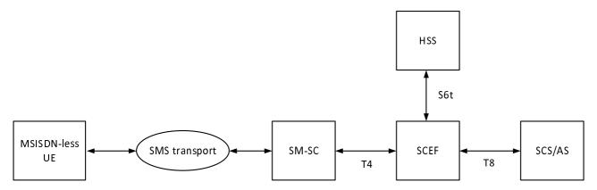
Figure 7.11-3: EPS architecture for MSISDN-less MO SMS
