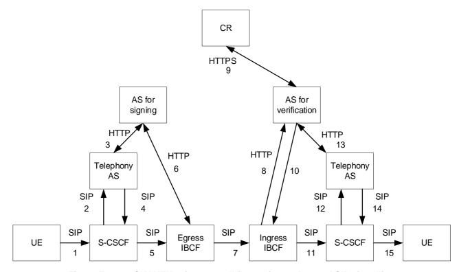
Figure E.4.1-1: SHAKEN reference call flow using end-to-end SIP signalling
