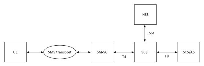
Figure 7.11-2: EPS architecture for device triggering
