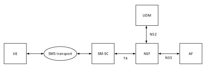
Figure 7.9-2: 5GS architecture for device triggering
