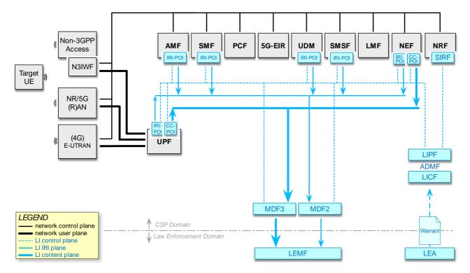
Figure 6.2-2: 5G core-anchored LI architecture
