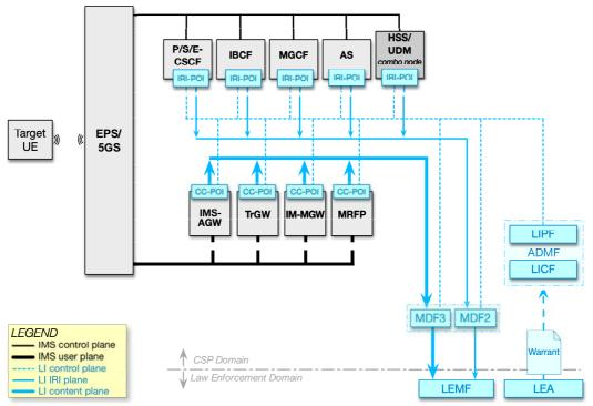
Figure 7.4-1: EPS/5GS-Anchored IMS High Level LI Architecture
