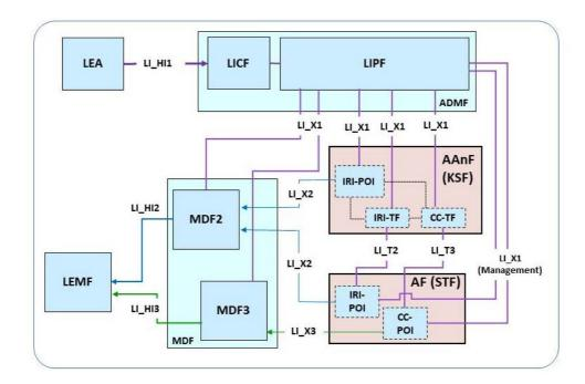
NOTE: If the AF is located outside the PLMN (not shown) the LI\_T2 and LI\_T3 interfaces are not used but LI\_X2 from IRI-POI in AAnF can still be used to provide IRI with key management information such as decryption keys via MDF2.
