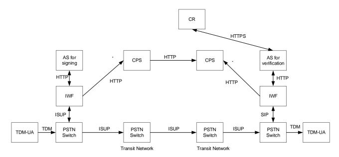
Figure E.2.4-2: Out of band SHAKEN reference architecture for end-to-end TDM signaling
