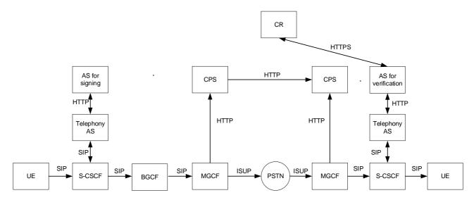
Figure E.2.4-1: Out of band SHAKEN reference architecture for non end-to-end SIP signaling
