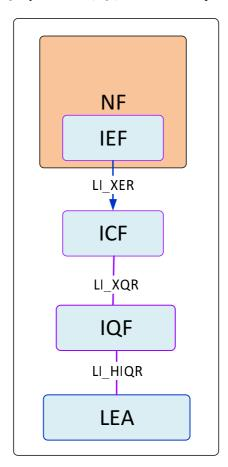
Figure 5.7-1 High-level identifier retrieval via Query and Response.
