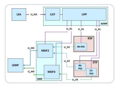
NOTE: If the STF is located outside the PLMN (not shown), the LI\_X2 from IRI-POI in KSF can be used to provide IRI with key management information such as decryption keys via MDF2.
