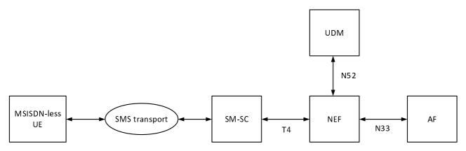
Figure 7.9-3: 5GS architecture for MSISDN-less MO SMS
