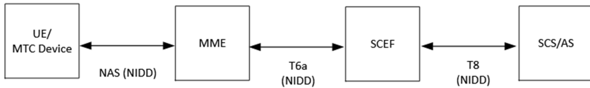
Figure 7.10-1: EPS Architecture for NIDD using SCEF
