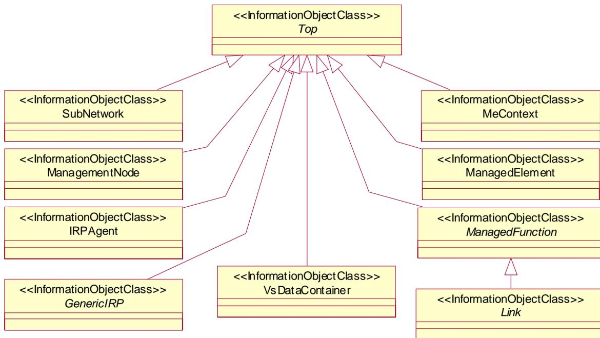
Figure 6.3: Generic Network Resource Model IRP Inheritance Hierarchy
