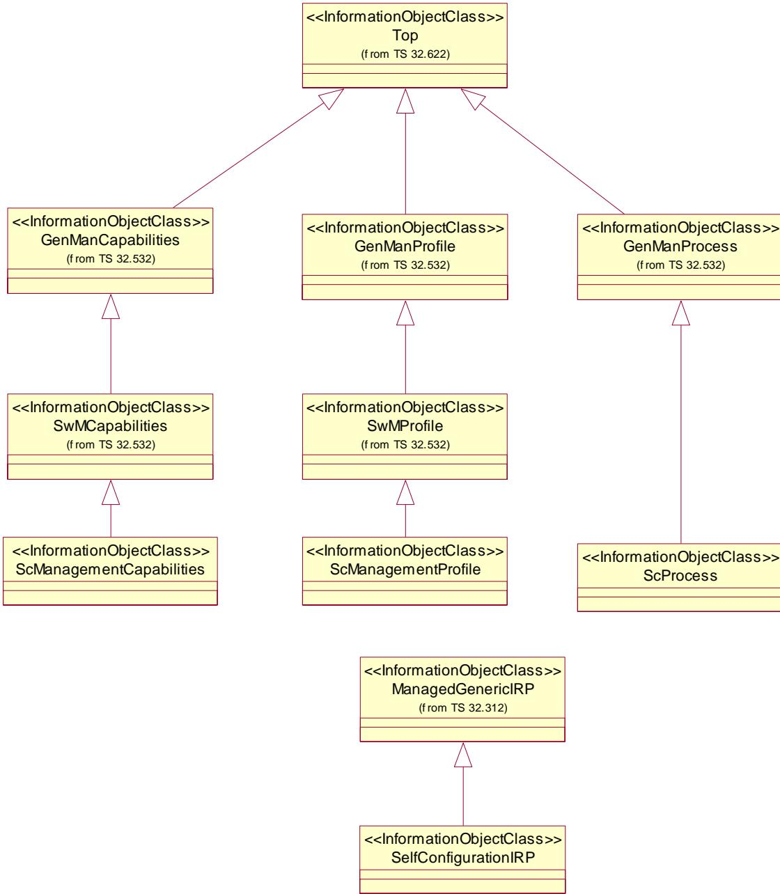
The following UML diagram describes the inheritance of the objects required for ARCF.
