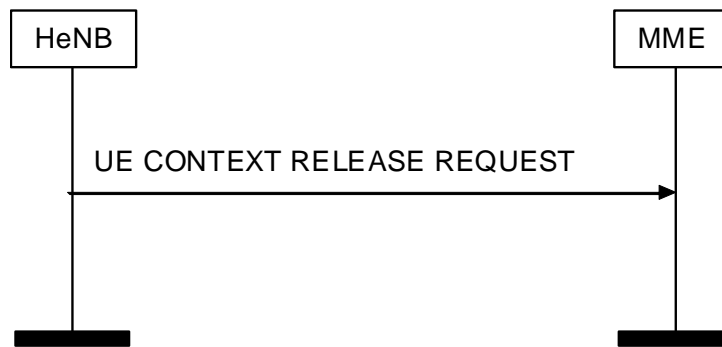
Figure 7 UE Context Release Request procedure. Successful operation
