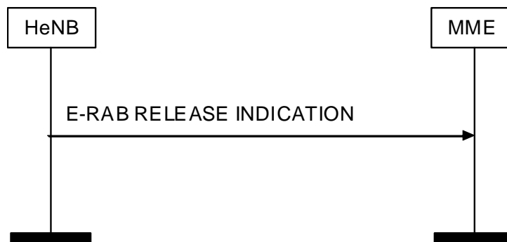
Figure 9 E-RAB Release INDICATION procedure. Successful operation
