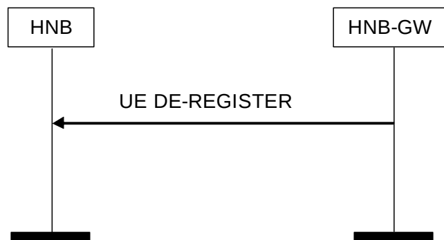
Figure 4 UE De-Register Procedure: HNB-GW Originated Successful Operation
