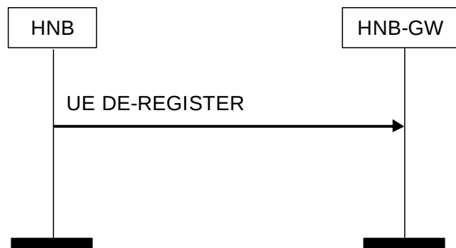
Figure 3 UE De-Register Procedure: HNB Originated Successful Operation
