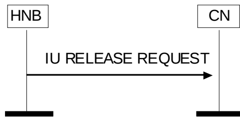
Figure 12 Iu Release Request procedure. Successful operation
