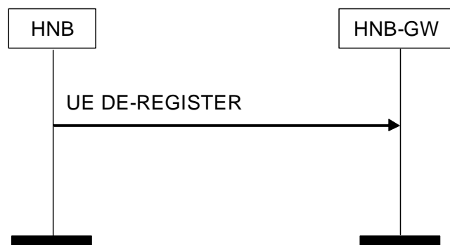
Figure 3 UE De-Register Procedure: HNB Originated Successful Operation
