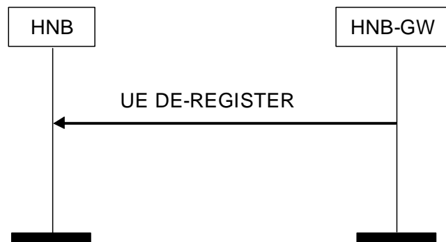
Figure 4 UE De-Register Procedure: HNB-GW Originated Successful Operation
