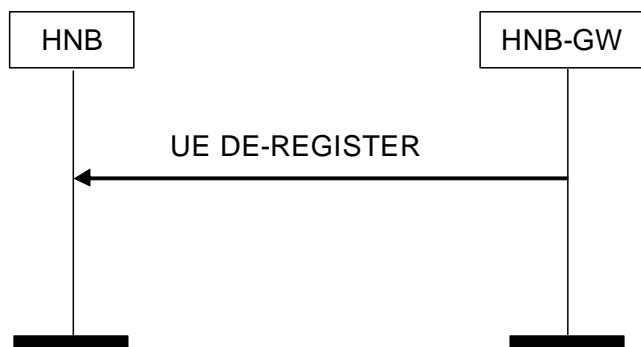
Figure 4 UE De-Register Procedure: HNB-GW Originated Successful Operation
