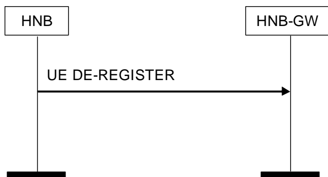
Figure 3 UE De-Register Procedure: HNB Originated Successful Operation
