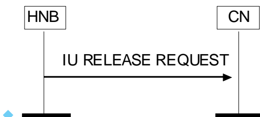
Figure 12 Iu Release Request procedure. Successful operation
