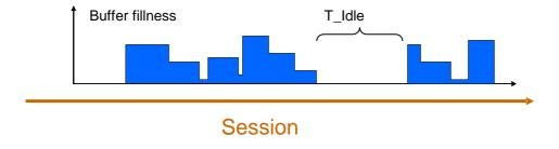
The measurements shall be defined so that impact of transport network problems are excluded (from the eNodeB this will just look like a bursty application since the transport network is not dimensioned to continuously fill the radio interface).
