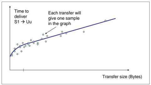
Hence, the measurement can be size dependent, unless care is taken, even if the performance of the eNodeB is the same in both cases. A method to exclude this is required.
