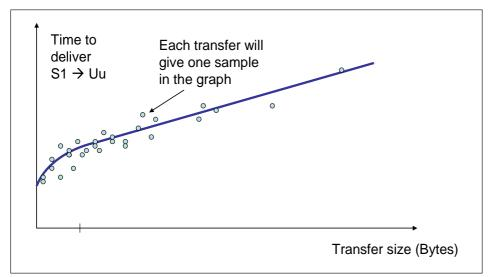
Hence, the measurement can be size dependent, unless care is taken, even if the performance of the eNodeB is the same in both cases. A method to exclude this is required.
