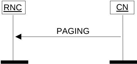
Figure: RANAP Paging procedure (Successful operation)
