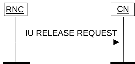
Figure: Iu Release Request procedure. Successful operation
