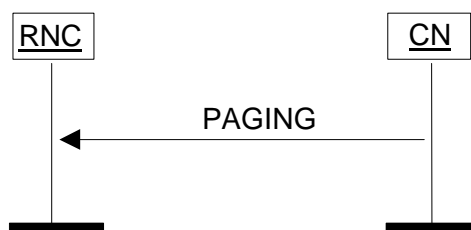
Figure: RANAP Paging procedure (Successful operation)
