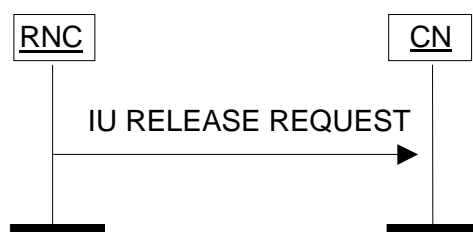
Figure: Iu Release Request procedure. Successful operation
