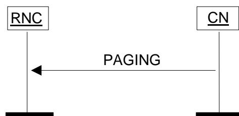
Figure: RANAP Paging procedure (Successful operation)
