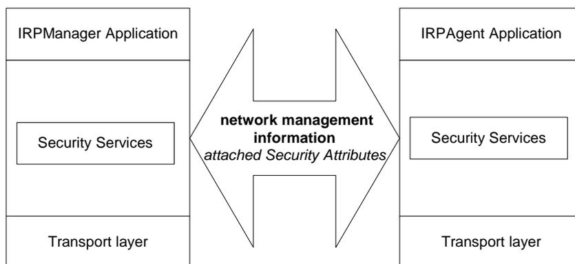
**Figure B.1 : Principles of IRP Security Service**
