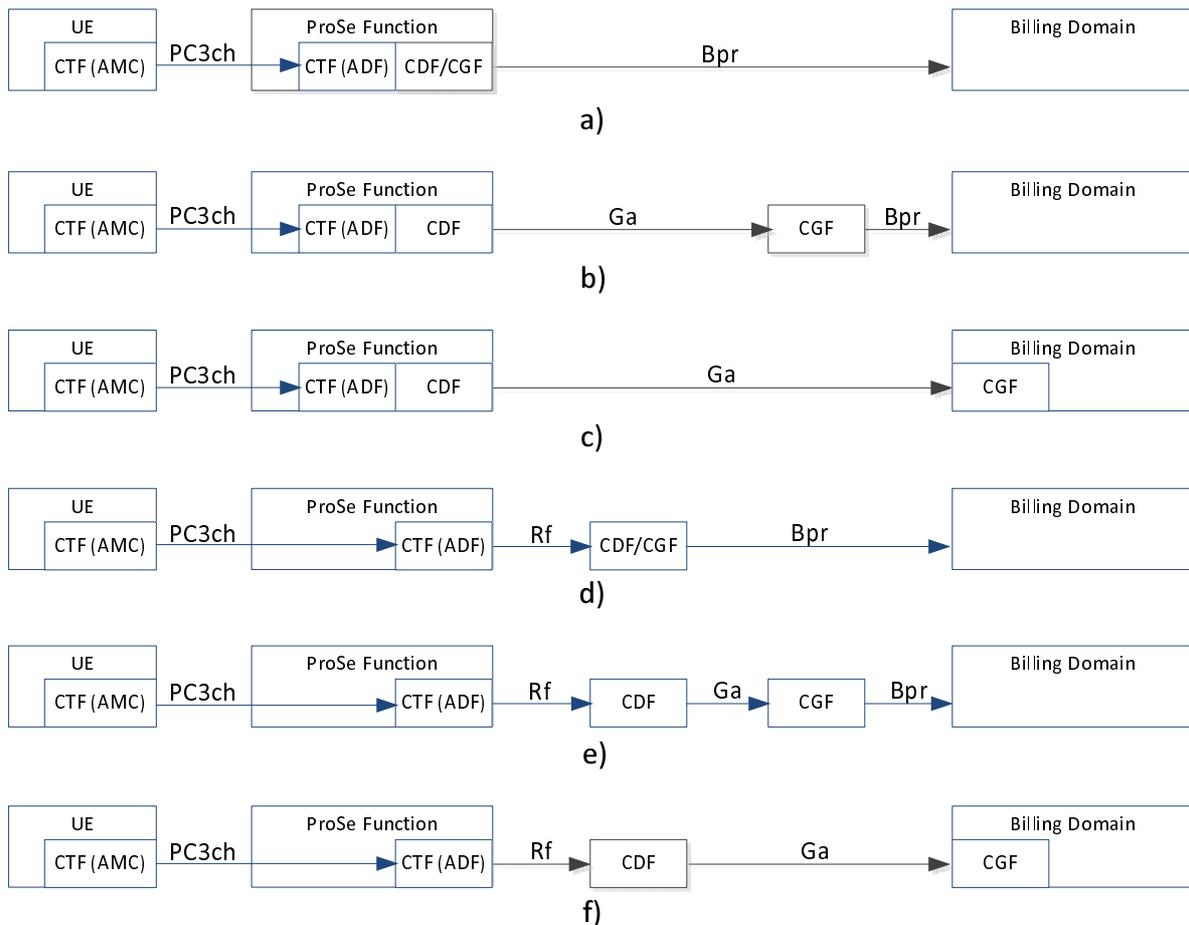
**Figure 4.2.2: ProSe Direct Communication offline charging architecture**
