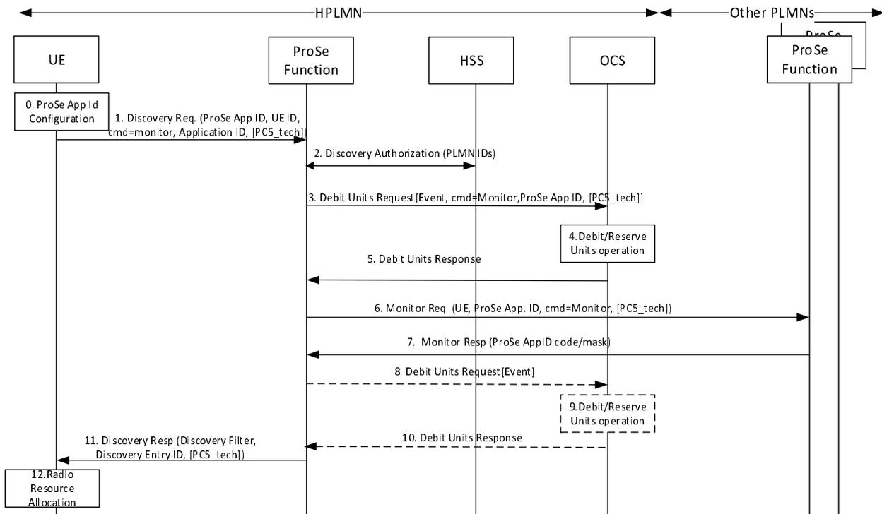
**Figure 5.3.2.2.3.1: ProSe Direct Discovery Monitor Request – IEC (non-roaming)**
