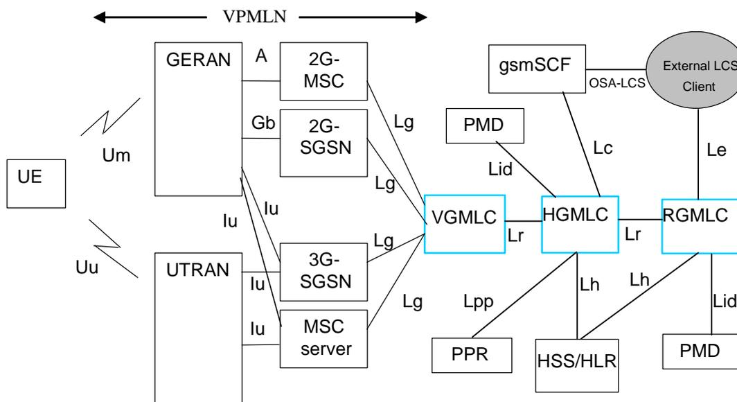
**Figure 4.1: LCS logical architecture with inter-GMLC [Lr] interface**
