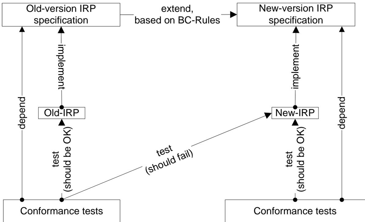
**Figure A.1: BC and Conformance Tests Scenario**
