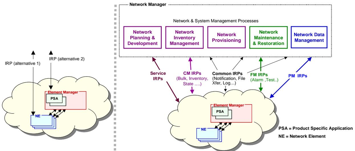
**Figure 4.3: Examples of IRPs for application integration**
