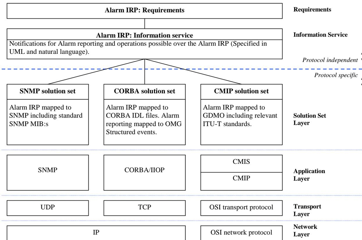
Figure 10.2: Example of an IRP (Alarm IRP)
