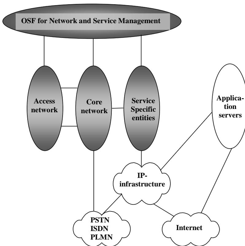
Figure 7.4 : High level UMTS Network architecture
