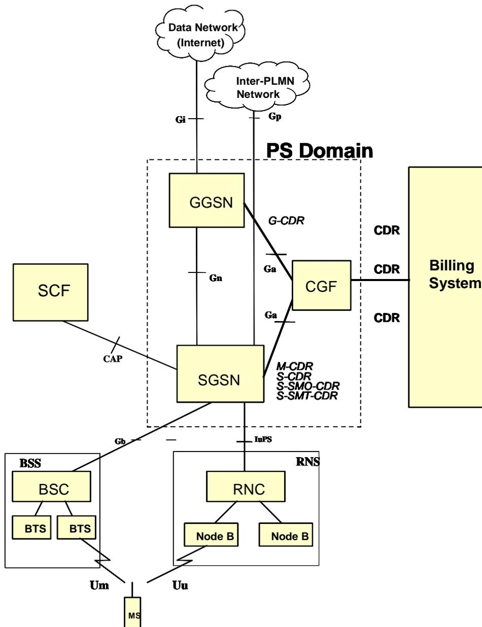
Figure 2: Packet Domain (PD) Charging logical architecture
