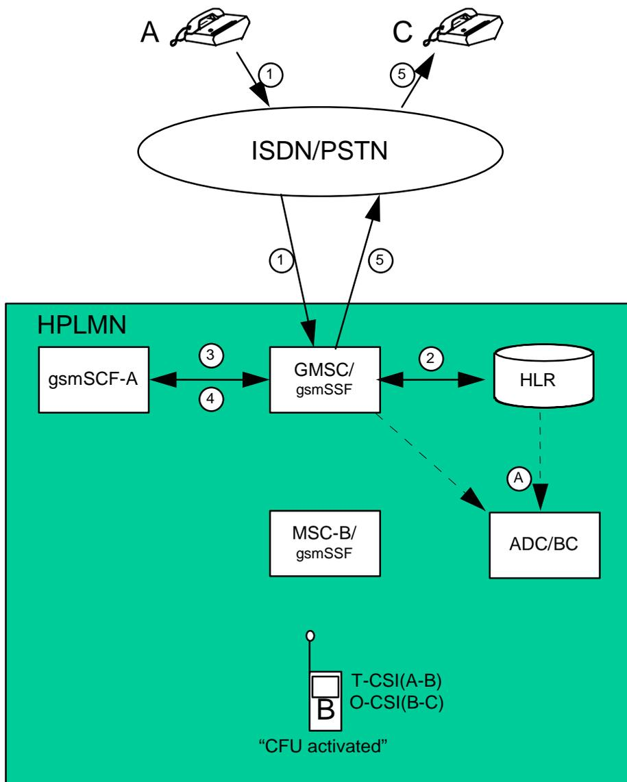
**Figure B.14: Incoming call handled by CAMEL without redirection and forwarded early using GSM SS but controlled by CAMEL**
