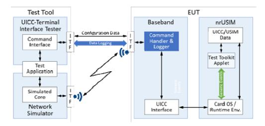
Figure 4.3: Test environment for seamless testing
