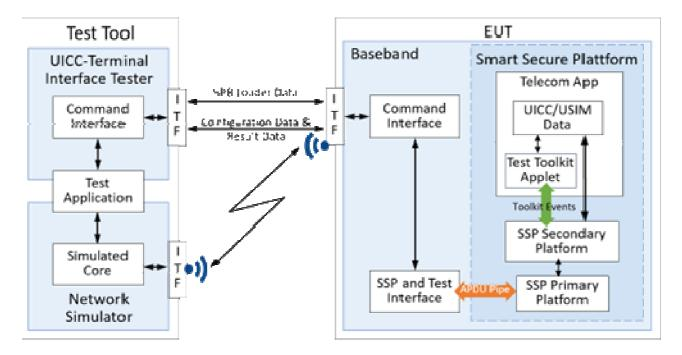
Figure 4.5: Test environment for UEs with ETSI eSSP/iSSP
