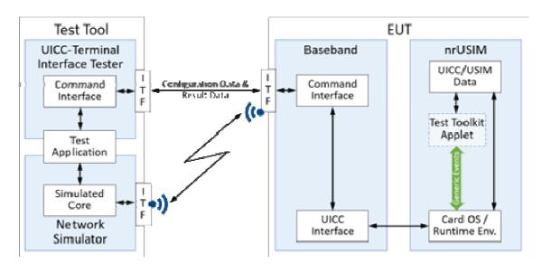
Figure 4.2: Test environment for implicit testing
