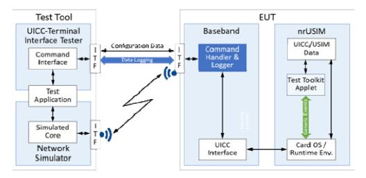
Figure 4.3: Test environment for seamless testing
