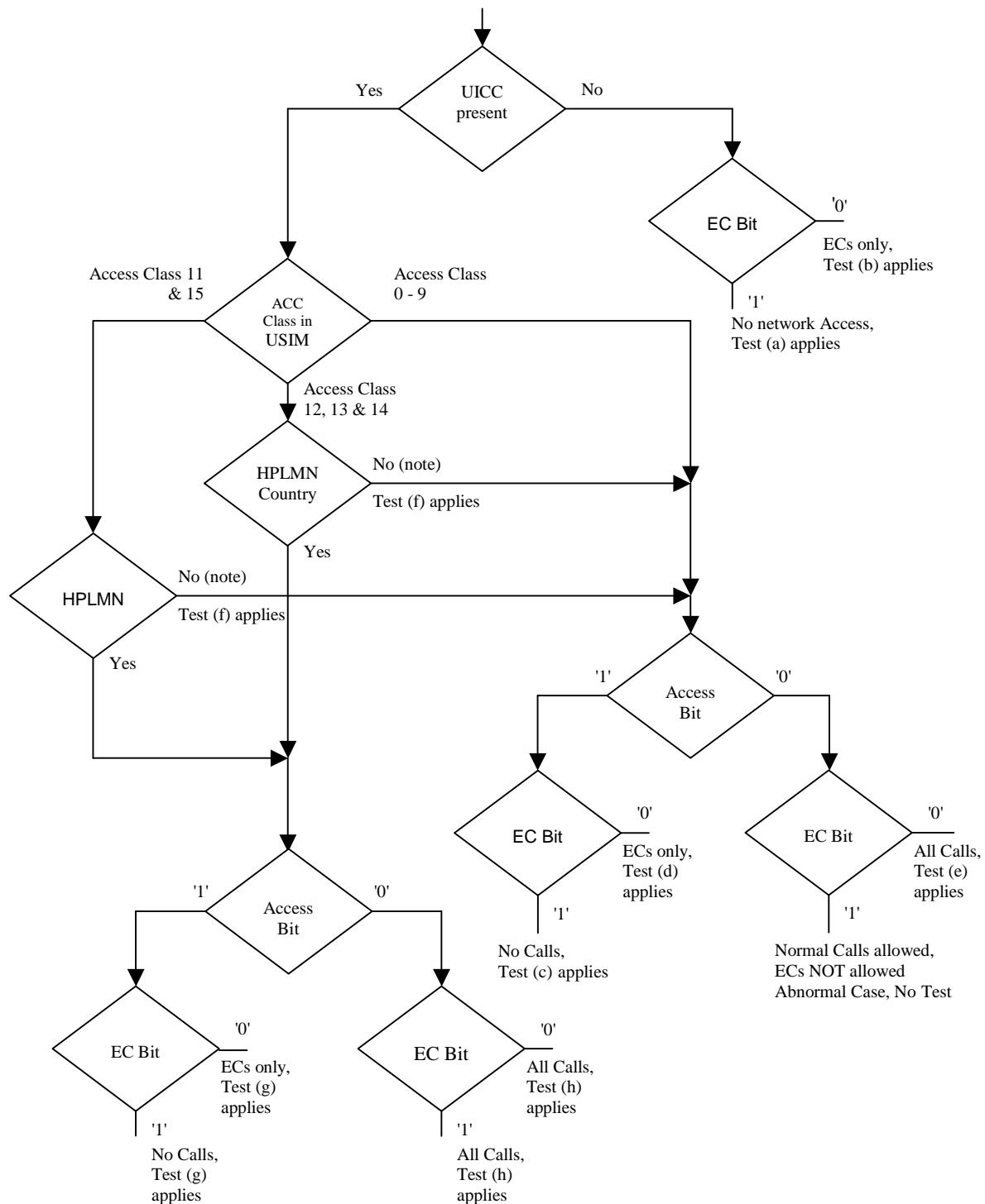
NOTE: UE adopts Access Class 0-9, based on IMSI, see TS 22.011. Access Class in USIM, See TS 31.102 EF ACC, "6F 78".
