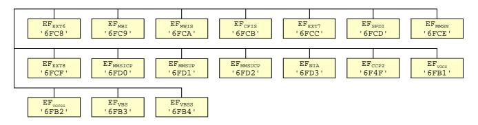
Figure 4.2: File identifiers and directory structures of USIM
