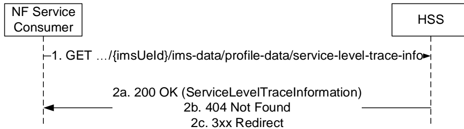
Figure 5.3.2.2.4.4-1: Service Trace Level Information Retrieval
