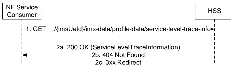
Figure 5.3.2.2.4.4-1: Service Trace Level Information Retrieval
