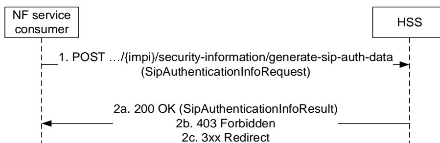
Figure 5.4.2.2.2-1: NF service consumer requesting authentication information
