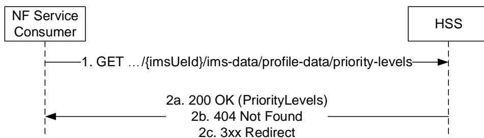
Figure 5.3.2.2.4.2-1: Service Priority Level Information Retrieval
