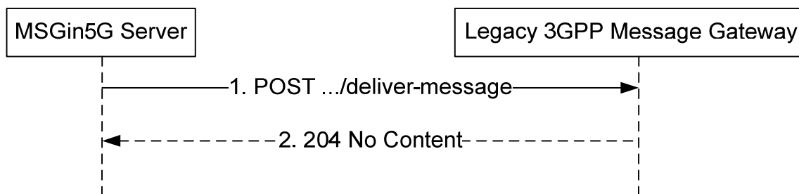
Figure 6.2.2.2.2-1: Legacy 3GPP Message Gateway Terminating Message Delivery
