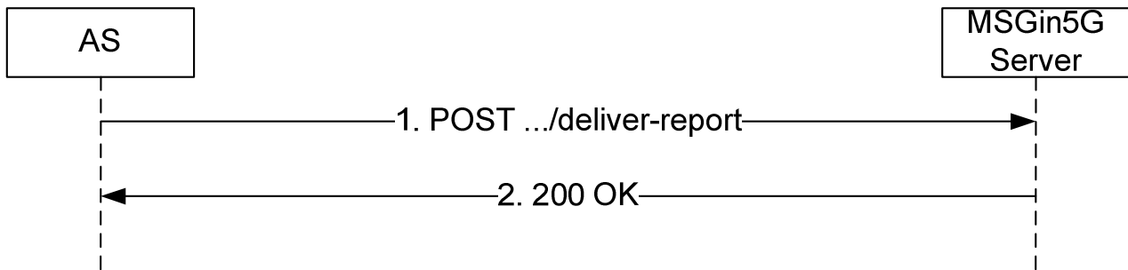
Figure 5.3.2.3.2-1: AS Originating MSGin5G Delivery Report
