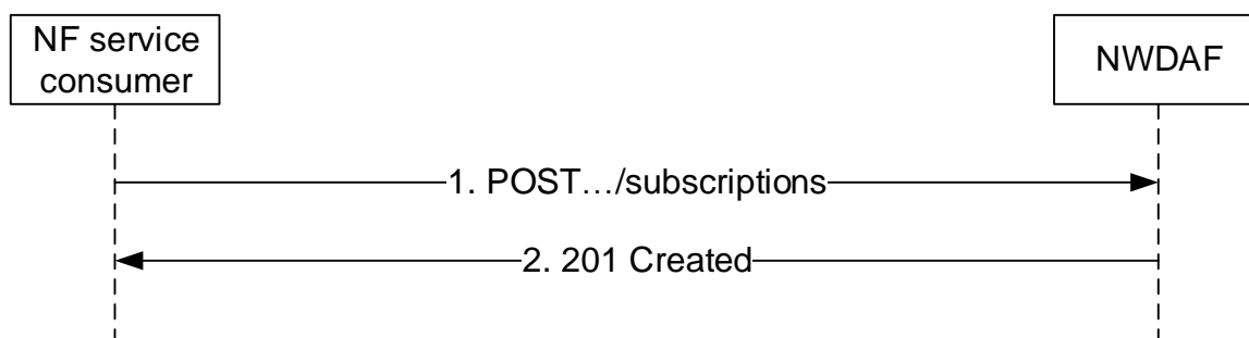
Figure 4.2.2.2.2-1: NF service consumer subscribes to notifications
